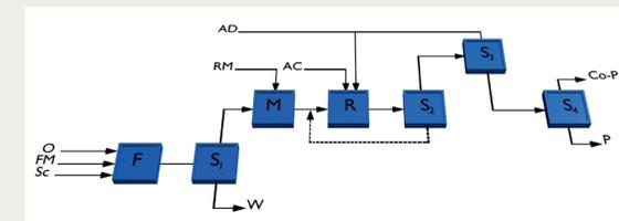
Different unit operations: fermenter (F), mixer (M), reactor (R) and separators (S1-4) can be arranged in the miniaturized platform and automatically screened. This gives the opportunity to rapidly screen for alternative reaction conditions (including reactant concentrations, product concentrations, fermentation media, pH conditions etc.).
